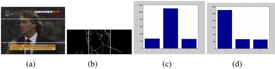
**Fig. 3.** Edge feature extraction (a) Partitioning the frame. (b) Partitioning the central slice and detecting the edges. (c) Obtaining the edge projection histogram. (d) Sorting the histogram.
