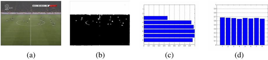
**Fig. 2.** Dominant color projection histograms (a) The original image. (b) The binary image. (c) The histogram of vertical axis projection. (d) The histogram of horizontal axis projection.
